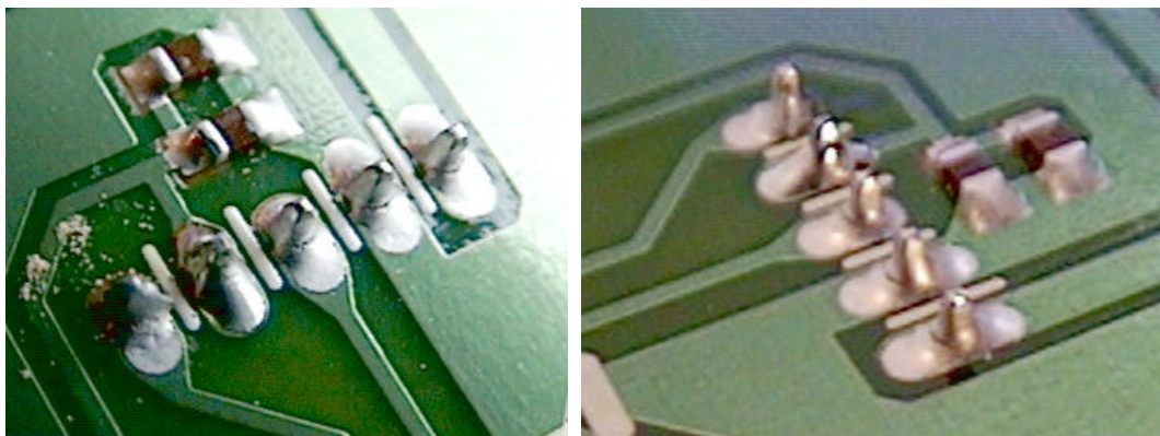
Bad pins may have a dull finish, and cracks as in these two pictures.
